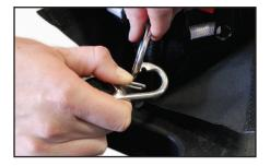
Take the clip end of the weight strap & secure to the center metal loop of the AirDome Leg.
